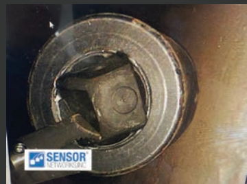
Large 1 in. drive impact socket retrieval with RGT
