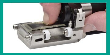
Despite the increasing use of adhesives as a joining technology for automotive body panels, adhesive bonding may not provide 100% process reliability. The Bond Scanner identifies areas with lack of adhesive, as well as misaligned bond lines, and provides a workflow-based, reliable inspection with the Mentor UT.
