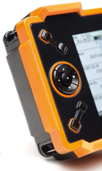
Introducing the new USM Go+ that takes field inspection NDT to the next level. Light, handy and controlled by an intuitive arrow-keypad, it has the latest industrial electronics under the hood and offers excellent ultrasonic performance which allows for reliable detection of defects located just below the surface of the test piece.
