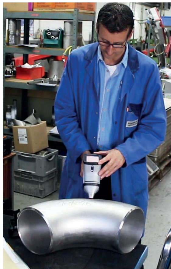
Non-destructive materials testing with the handheld XRF X-MET8000
